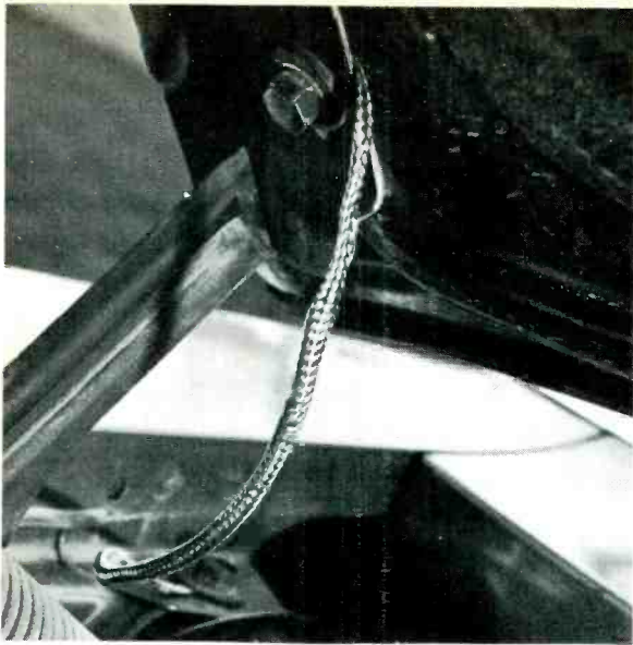
Fig. 5 Hood hinges often are not a good ground to RF and noise. Add a ground of braided shielding at each side hinge.
